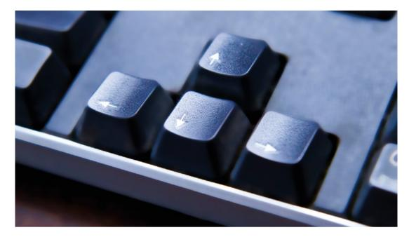
To respond to key presses, Pygame Zero has a builtin object called keyboard. The arrow kev states can be read with keyboard. up, keyboard.down and so on
