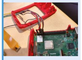
A Raspberry Pi 3B+ was used to trigger the water spray, lights, and fans, bringing an extra element to the gameplay, as well as rendering the arcade machine's graphics.
