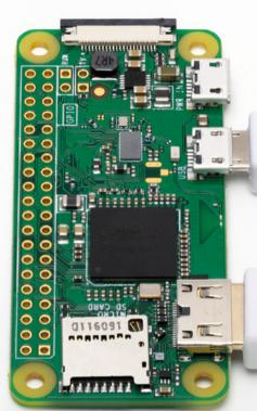
Raspberry Pi Zero W features a mini-HDMI socket. You'll need a mini-HDMI to full-sized HDMI adapter like this to connect your Raspberry Pi Zero W to an HDMI display
