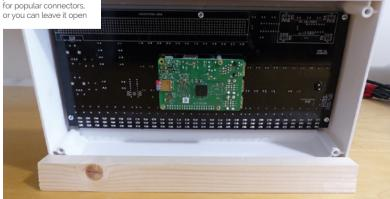
Once built, the PiDP-11 PCB comprises 64 LEDs, two rotary encoders, and an array of switches that connect to Raspberry Pi's GPIO. Running a special version of the SimH emulator, Raspberry Pi accurately handles input and output from the panel. You can hook up a screen, use SSH, or go old-school and implement RS-232. The back panel has different cut-outs to suit your cabling.
