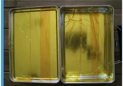
One obvious problem with using a metal box is its conductivity, so to avoid any possibility of short circuits, Daniel lined it with Kaplon insulating tape before adding the electronics.
