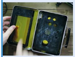
After careful measuring, Daniel designed and 3D-printed a screen holder, which he hot-glued to the lunchbox lid, and a board to house the arcade controls and speaker.
