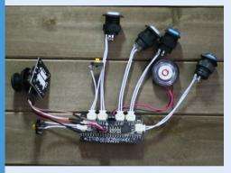
The analogue thumb joystick, six buttons, and 0.25 W 8  $\Omega$  speaker were connected to an Adafruit Arcade Bonnet. A couple of freely available scripts were then run to get everything working.
