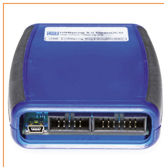
Figure 2. The USBprog 5.0 connections. To the right a 14-pin Gnuclin/EEC connector; A future firmware update will allow control of Gnuclin expansion boards.
