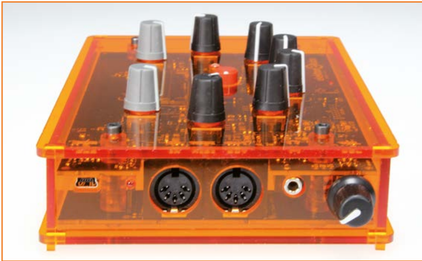
Figure 6. The J 2 B synthesizer in a laser-cut Plexiglass enclosure.
