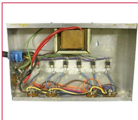
Figure 3. The remote box contained the triacs to switch the lights. At the bottom are the sockets for connection to the light bars; the console cable plugged into the socket on the bottom left. The transformer supplied stepped down AC to the console.
