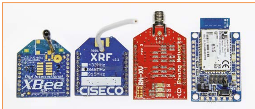
Figure 1. Several wireless modules from Digi, Ciseco and Microchip. All of them fit T-Board Wireless.
