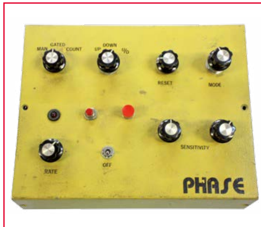
Figure 1. The console manages the operation of the light show; the wear and tear seen here shows the console was used quite often. In the lower right corner, PHASE is the identity I used when working sound and lights for the dance gigs.
