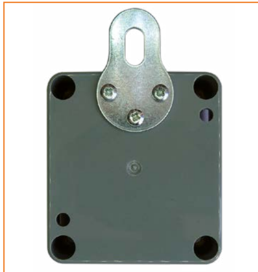
Figure 5. The author's prototype, in a waterproof case and fitted with a sturdy screwed hook.
