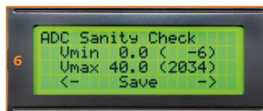
Figures 1 to 6. The various menus displayed on the LCD: (1) Start-up screen; (2) Home page; (3) Setup, (4) Calibration 1; (5) Calibration 2; (6) Status.
